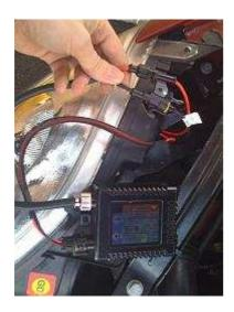
Take one of the supplied Ballasts and connect the dual connector making sure the black is lined up with the negative position on the ballast!!. Now connect the positive and negative to the correct wires to the rear of your headlight, making sure that they are secure.
