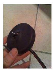
Push the HID loom through and secure with the rubber bung supplied with the loom.
